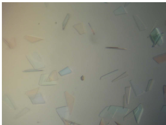
Figure 1 Typical thin plate-shaped crystals of N -acetyl-L-citrulline deacetylase. The largest dimension was approximately 0.4 mm.
